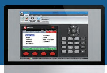
**OMNIPANEL®** is another feature that makes the OMNI 4000/7000 user friendly. OMNI-PANEL is a convenient, Windows-based software application that delivers the look and function of the OMNI 4000/7000 front panel via a software interface.
